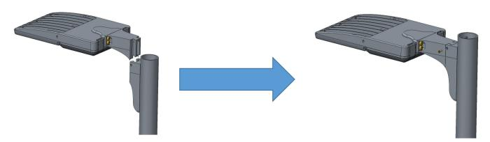
Step4: Wiring, connect the L,N,GND wires on the lamp to the correspondingL,N,GND cables on the pole.
